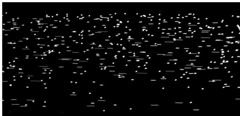
Figure 3. Particle streak image for 500 \mu\text{m} microchannel, using 200 ms exposure time.
